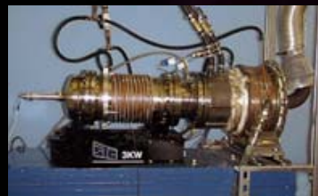
Above: ARL's Stirling engine for nuclear power conversion.
